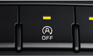
Idle Stop & Go system (ISG) ISG reduces fuel consumption by automatically shutting down the engine when the vehicle is at a standstill.
