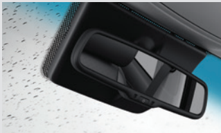
Rain sensor The rain sensor detects raindrops on the windshield and activates the wipers when a coverage threshold is met.
