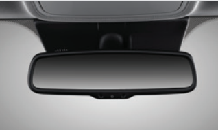
ECM rear-view mirror At night, the Electro-Chromic Mirror automatically controls the glare from the headlamps of the car behind you.
