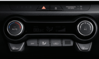
Full Automatic Air Conditioner (FATC) FATC offers set-and-forget functionality, automatically turning the system on and off to maintain the desired temperature in the cabin.
