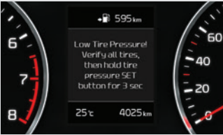
Indirect TPMS Using the ABS system's wheel speed sensors, indirect TPMS detects air loss in tyres through differences in relative wheel speeds.
