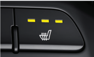
Heated front seats Heated front seats include three adjustable warmth levels to keep you cosy when it's chilly outside.
