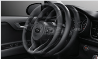
Telescopic and tilt steering Adjust the steering column up and down, and in and out, to find just the right position for you.
