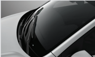
Aero blade wipers Aerodynamic wiper blades keep the blade in contact with the windshield at high speeds.
