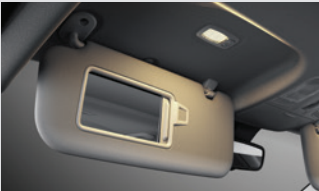
Sun visor illumination lamps LED lights beside the vanity mirror on the driver-side sun visor light up to help you check your appearance in the mirror.
