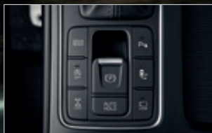
Drive Mode Select (DMS) The new automatic transmission allows you to choose between four different drive modes: Eco, Comfort, Sport and Smart. Each mode lets you customise the power train's responses to driver inputs, enhancing fuel economy or acceleration. The Drive Mode Select system also adapts the weight of the rack-mounted power steering system, for more relaxed or more immediate, engaging steering responses.
