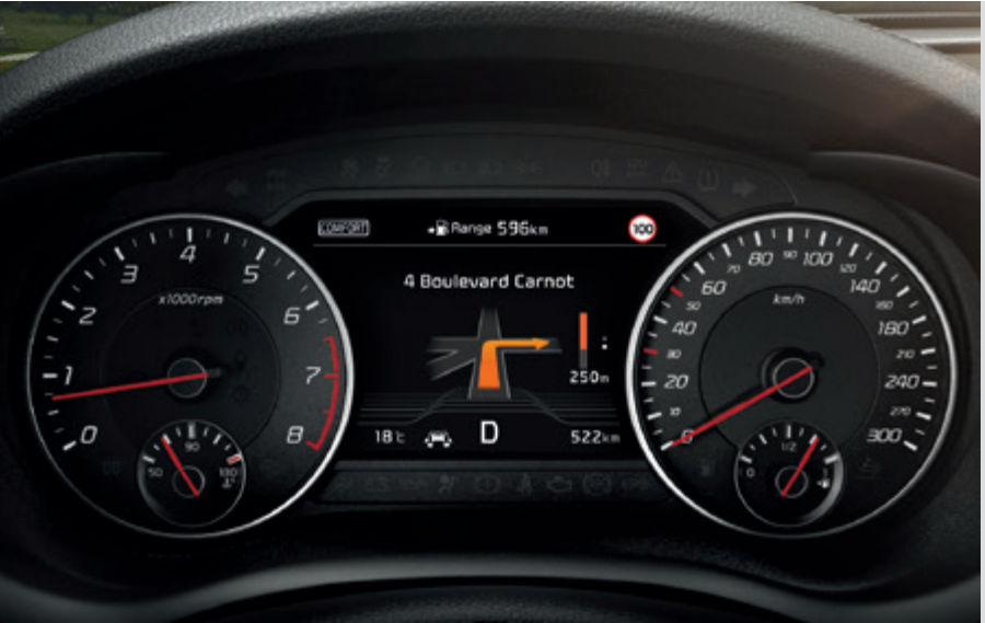
7" screen supervision cluster The high-definition 7-inch TFT LCD in the supervision cluster provides customisable data essentials – from average fuel economy to turn-by-turn navigation information.
