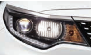
Single projection-type headlamp with LED DRLs (LX)
