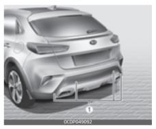
Forward/Reverse Parking Distance Warning system assists the driver during movement of the vehicle by chiming if any object is sensed within the distance of 100 cm (40 in) in front and 120 cm (48 in) behind the vehicle.
