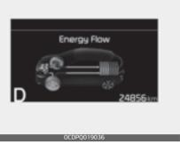
The engine compression can be used to slow the vehicle. The regenerative braking system can be used to charge the hybrid system.
