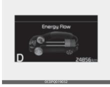
Hybrid battery is being charged by regenerative braking.
