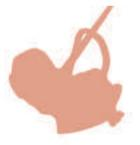
A rearward-facing Child Restraint System provides restraint with the seating surface against the back of the child. The harness system holds the child in place, and in an accident. acts to keep the child positioned in the Child Restraint Systems and reduce the stress to the fragile neck and spinal cord.
