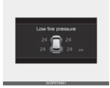
When the tire pressure monitoring system warning indicators are illuminated and warning massage displayed on the cluster LCD display, one or more of your tires is significantly under-inflated. The low tire pressure position telltale light will indicate which tire is significantly under-inflated by illuminating the corresponding position light.
