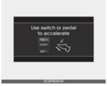
While Smart Cruise Control system is in operation, your vehicle stops behind the vehicle in front when it stops. The message is displayed on the cluster within 3 seconds after the stop and the system will be in the standby position.
