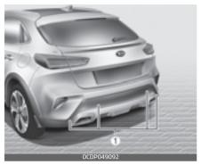
Reverse Parking Distance Warning system assists the driver during reverse movement of the vehicle by chiming if any object is sensed within the distance of 120 cm (48 in) behind the vehicle.
