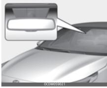
When the system detects the vehicle straying from its lane or road, it alerts the driver with a visual and audible warning, while applying a slight counter-steering torque, trying to prevent the vehicle from moving out of its lane or road.
