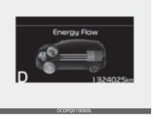
Engine is both driving the vehicle and charging the hybrid battery.
