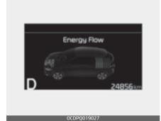
The mode means the vehicle is stopped. (There is no energy flow.)
