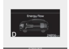
The vehicle is being slowed down by engine compression and regenerative braking. The hybrid battery is being charged by regenerative braking.
