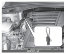
In case of emergency, cut the service interlock connector cable to isolate the high voltage of the battery.
