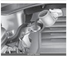
If it is near or at L (Low), add enough oil to bring the level to F (Full). **Do not overfill**.
