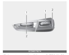
If the stop and tail lamp (LED) (1,2) does not operate, have your vehicle checked by a professional workshop.
