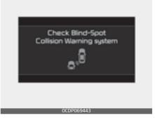
If the system does not work properly, a warning message will appear and the light on the switch will turn off. The system will turn off automaticallu.
