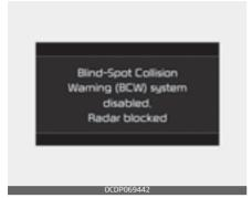
The message will appear to notifu the driver if there are foreign substances on the surface or inside the rear bumper or it is hot near the rear bumper. The light on the switch and the system will be turned off automaticallu.
