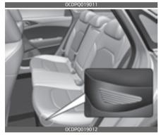
The hybrid battery air intake is located on bottom and side of the rear seats. The air intake cools down the hybrid battery. When the hybrid battery air intake is blocked, the hybrid battery may be overheated. Do not obstruct the air intake with any other objects.
