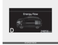
The engine and regenerative braking system charge the hybrid battery driving deceleration.
