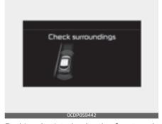
Parking Assist checks the front and rear space to exit the vehicle from the parking space.
