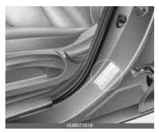
All specifications (sizes and pressures) can be found on a label attached to the vehicle.
