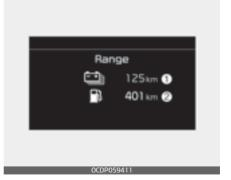
The range is the estimated distance the vehicle can be driven with the remaining high-voltage (hybrid) battery (1, Electric) and fuel in the fuel tank (2, Gasoline).
