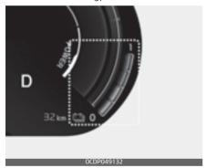
This gauge indicates the remaining hybrid battery power. If the SOC is near the "L (Low) or 0" level, the vehicle automatically operates the engine to charge the battery. However, if the Service Indicator ( ) and Malfunction Indicator Lamp (MIL) (X) turn on when the SOC gauge is near the "L (Low) or 0" level, have the vehicle checked by a professional workshop. Kia recom-
