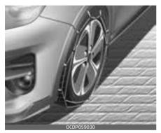
Since the sidewalls of radial tires are thinner, they can be damaged by mounting some types of snow chains on them. Therefore, the use of snow tires is recommended instead of snow chains. Do not mount tire chains on vehicles equipped with aluminum wheels; snow chains may cause damage to the wheels. If snow chains must be used, use wire-type chains with a thickness of less than 12 mm (0.47)
