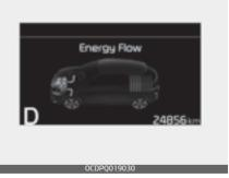
Engine power is used to move the vehicle.
