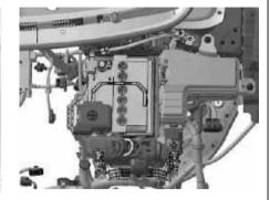
3. Battery in the engine compartment
