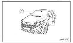
The Traffic Sign Recognition (TSR) system provides the driver with information about the most recently detected speed limit. The system captures the road sign information with the front camera unit (1) located in front of the interior rear-view mirror and displays the detected signs in the Vehicle Information Display and in the Head Up Display (HUD) (where fitted).
