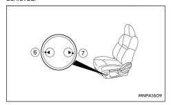
Power adjustment (where fitted): Push each side of the adjusting switch to adjust the seat lumbar area until the desired position is achieved
