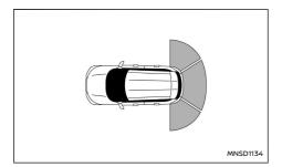
The parking sensor (sonar) system sounds a tone to inform the driver of obstacles near the rear bumper.
