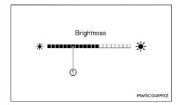
The instrument brightness control switch can be operated when the ignition is ON. When the switch is operated, the vehicle information display switches to the brightness adjustment mode.
