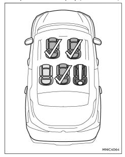
In vehicles fitted with Rear Occupant Detection, in addition to the Seat Belt Warning Light, the Occupant Status Display will be shown in the Vehicle Information Display (See "Vehicle information display" (P.80).) when any vehicle occupant's seat belt is not fastened.
