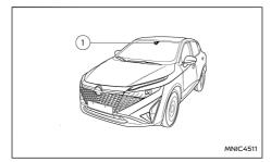
The lane camera unit (1) for the Traffic Sign Recognition (TSR) system is located above the interior rear view mirror. To maintain the proper operation of the Traffic Sign Recognition (TSR) system and prevent a system malfunction, be sure to observe the following:
