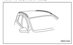
Luggage can be carried on the roof by securing crossbars to the roof rail. Follow all crossbar manufacturers instructions for installing and use of the crossbars. The roof rail is designed to carry loads (luggage plus crossbars) below 75 kg (165 lb). Overloading may cause damage to the vehicle.
