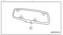
The inside mirror is designed so that it automatically adjusts the reflection according to the intensity of the following vehicle's headlights on the sensor (A).
