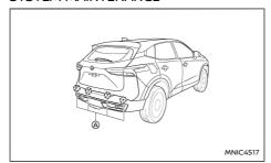
The parking sensor (sonar) sensors (A) are located on the rear bumper.
