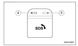
The indicator lights (4) and (5) above the <SOS> button indicate the status of the vehicle emergency call system. If the indicator light is illuminated red or no indicator light is illuminated the emergency call may not connect to the emergency call centre when the <SOS> button is pressed. Also an automatic emergency call may not be sent when a collision occurs
