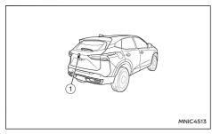
To display the rear view, the Rear-view Monitor system uses a camera ① located just above the vehicle's number plate.
