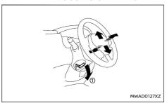
Pull the lock lever (1) down and adjust the steering wheel up, down, forward or rearward to the
