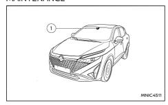
The lane camera unit (1) for the Traffic Sign Recognition (TSR) system is located above the interior rear view mirror. To maintain the proper operation of the Traffic Sign Recognition (TSR) system and prevent a system malfunction, be sure to observe the following:
