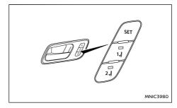
Two positions for the driver's seat can be stored in the Driving Position Memory System memory. Depending on vehicle specification, it may also be possible to store the position of outside mirrors. Follow these procedures to use the memory system.
