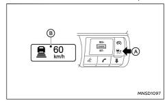
To turn the cruise control on, quickly push and release the ICC switch (A). The ICC system ON indicator (grey), and set vehicle speed indicator ---(B) come on.
