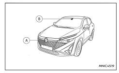
The sensor (A) is located at the front of the vehicle.
