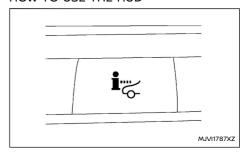
To turn the HUD on, push the HUD switch. To turn the HUD off, push the switch again.
