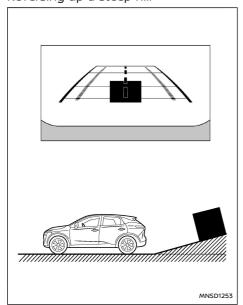
When reversing a vehicle up a hill, the distance guide lines and the vehicle width guide lines are shown closer than the actual distance. Note that any object on the hill is viewed in the monitor further than it appears.
