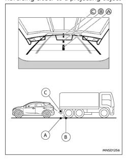
The position © is shown further than the position ® in the display. However, the position © is actually at the same distance as the position ®. The vehicle may hit the object when moving toward the position ® if the object projects over the actual moving course.
