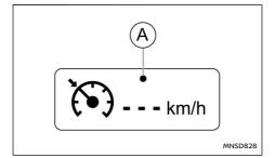
When pushing the ICC ON/OFF switch on, the ICC system display and indicators are displayed in the vehicle information display. After you hold the ICC ON/OFF switch for longer than about 1.5 seconds, the ICC system display goes out. The cruise indicator appears. You can now set your desired cruising speed. Pushing the ICC ON/OFF switch again will turn the system completely off.
