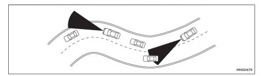
When driving on some roads, such as winding, hilly, curved, narrow roads, or roads which are under construction, the radar sensor may detect vehicles in a different lane, or may temporarily not detect a vehicle travelling ahead. This may cause the I-FCW system to work inappropriately.
