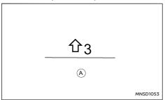
The shift indicator (A) located in the lower part of the vehicle information display can help to improve the level of environmentally friendly driving. Following the shift indicator by changing to the suggested gear when displayed may improve fuel economy.
