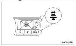
The distance to the vehicle ahead can be selected when the ICC is in standby mode or the ICC is active, depending on the traffic conditions.
