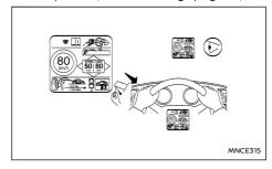
4. Remove the speed restriction sticker from the compressor, then place it in a location where the driver can see it while driving.
