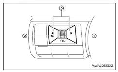
The vehicle information display can be changed using the scroll dial ①, **5** ②, and **4 b** ③ located on the steering wheel.
