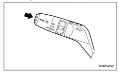
To activate the high beam assist system, push the switch as illustrated when it is in the <AUTO> position. The high beam assist indicator light in the instrument panel will illuminate.
