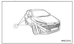
To display the multiple views, the Intelligent Around View Monitor system uses cameras ① located on the front grille, on the vehicle's outside mirrors and one just above the vehicle's rear number plate.
