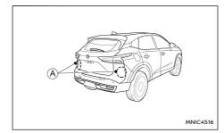
The two radar sensors (A) for the BSW system are located near the rear bumper.
