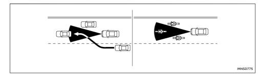
The detection zone of the radar sensor is limited. A vehicle ahead must be in the detection zone for the vehicle-to-vehicle distance detection mode to maintain the selected distance from the vehicle ahead.
