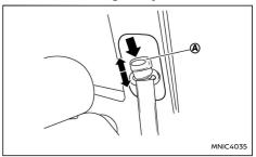
The shoulder belt anchor height should be adjusted to the position that is best for you. (See "Precautions on seat belt usage" (P.25).)
