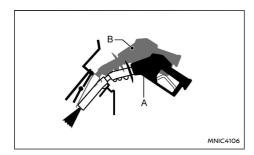
Hold the fuel pump nozzle in position A (shown). Holding the fuel pump nozzle in position B may cause fuel pump nozzle to shut off before the tank is full.
