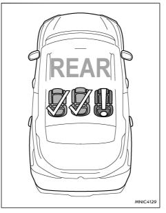
In vehicles not fitted with Rear Occupant Detection, the Rear Passenger Seat Belt Display will be shown in the Vehicle Information Display (See "Vehicle information display" (P.80)) for approximately 65 seconds when the ignition is switched ON while any rear seat belt is unfastened. The driver can acknowledge the display by pushing the **<OK>** steering wheel switch.
