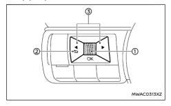
Switches for the vehicle information display are located on the left side of the steering wheel.
