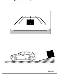
When reversing a vehicle up a hill, the distance guide lines and the vehicle width guide lines are shown closer than the actual distance. Note that any object on the hill is viewed in the monitor further than it appears.
