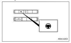
When the system malfunctions, it turns off automatically. The Steering Assist status warning illuminates (vellow) and a warning message is displayed in the vehicle information display. A chime may sound depending on the situation.
