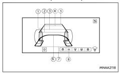
The invisible hood view allows the user to see the road surface under the virtually transparent vehicle body. This my be useful for aligning the front wheels with the rails of an automatic car wash, or to avoid hitting the side of the vehicle against kerbs when operating at low speeds, for example.
