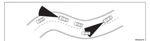
When driving on some roads, such as winding, hilly, curved, narrow roads, or roads which are under construction or on a slope, the sensor may detect vehicles in a different lane, or may temporarily not detect a vehicle travelling ahead. This may cause the system to work inappropriately.
