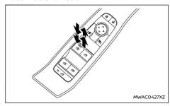
The automatic function enables a window to fully open or close without holding the switch down or
