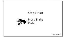
This guidance is displayed when the vehicle is stopped if the Stop/Start System is deactivated due to not fully depressing the brake pedal.
