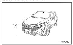
The radar sensor is located on the front of the vehicle (A).
