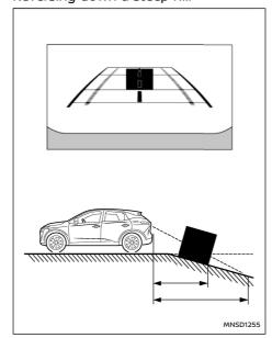
When reversing the vehicle down a hill, the distance guide lines and the vehicle width guide lines are shown further than the actual distance. Note that any object on the hill is viewed in the monitor closer than it appears.
