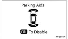
When the vehicle is in R (Reverse) and the [Parking Aids] screen is displayed in the vehicle information display the RAB system can be disabled temporarily by pushing the <OK> switch on the steering wheel.
