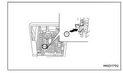
To reduce battery drain, the extended storage fuse switch (1) comes from the factory switched off. Prior to delivery of your vehicle, the switch is pushed in (switched on) and should always remain on.
