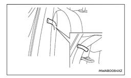
2. When folding the rear seat forward, the outer seat belts can be stored out of the way using the seat belt hooks as shown in the illustration.
