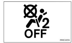
If the child restraint is installed on the front passenger seat, switch the ignition ON. The <PASSENGER AIR BAG OFF> | light, located on the roof console, should illuminate. If the <PASSENGER AIR BAG ON> | light is illuminated, see "Supplemental Restraint System (SRS)" (P.49). Move the child restraint to another seating position. Have the system checked by a NISSAN dealer or qualified workshop.
