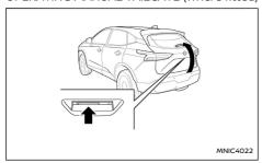
To open the tailgate, unlock it. Pull up the tailgate to open.
