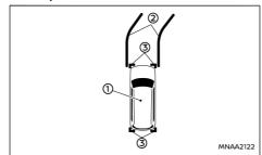
The bird's-eve view shows the overhead view of the vehicle which helps confirm the vehicle position and the predictive course to a parking space.
