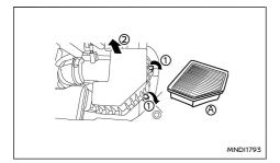
cleaning or replacing the filter, wipe the inside of the air cleaner housing and the cover with a damp cloth.
