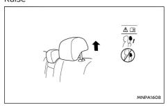
To raise the head restraint, pull it up as shown.
