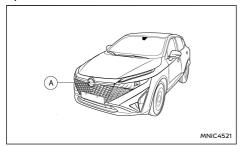
The sensor for the ICC system is located on the front of the vehicle (A)
