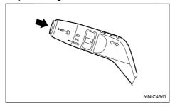
To switch on the Adaptive Driving Beam system. push the switch as illustrated when it is in the <AUTO> position. The Adaptive Driving Beam indicator light  $\equiv (A)$  in the instrument panel will illuminate.
