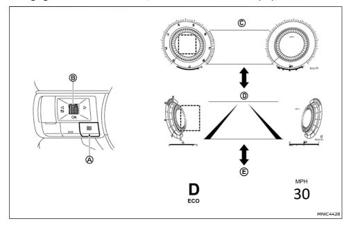
For models with full-screen display, the meter screen view can be changed between [Normal] ©, [Enhance] (D) and [Minimal] (E) views.
