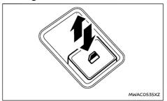
The passenger's switch can control its corresponding window. When the window lock button on the driver's switch is pushed, rear passenger's switches cannot be operated, but the front passenger's switch can still be operated.
