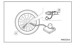
5. Screw the air tube (A) of the compressor securely onto the tyre valve. Make sure that the air compressor switch is in the OFF position and the pressure release valve (B) is securely closed.
