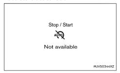
If the engine stops when the Stop/Start System is activated, and will not start automatically, the message is shown.
