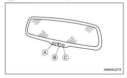
The inside mirror is designed so that it automatically adjusts the reflection according to the intensity of the following vehicle's headlights on the sensor O.
