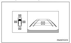
When the "\sqrt{" icon is displayed on the screen, the camera image may be receiving temporary electronic disturbances from surrounding devices. This will not hinder normal driving operation but the system should be inspected. It is recommended you visit a NISSAN dealer or qualified workshop.
