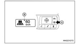
To turn the cruise control on, quickly push and release the Drive Assist switch (A). The ICC system ON indicator (grey), and set vehicle speed indicator (B) come on.
