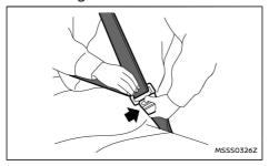
To unfasten the seat belt, push the button on the buckle. Then guide the seat belt as it automatically retracts
