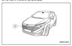
The sensor (a) is located at the front of the vehicle.
