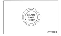
When the ignition switch is pushed without depressing the brake pedal, the ignition switch will illuminate:
