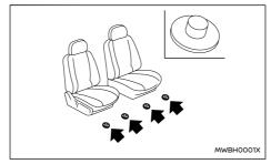
This vehicle includes front floor mat brackets A to act as a floor mat positioning aid. Genuine NISSAN floor mats have been specially designed for your vehicle
