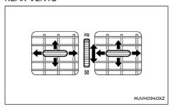
Open/close the vents by moving the control to either direction.
