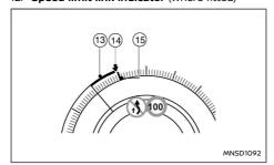
13. Green line: Intelligent Cruise Control (ICC) (where fitted): gap between current speed and ICC target speed.
