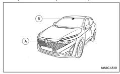
The IEB system uses a radar sensor (a) located on the front of the vehicle and camera (b) installed behind the windscreen in to measure the distance to the vehicle, pedestrians and cyclists ahead in the same lane (where pedestrian or pedestrian and cyclist detection is fitted).
