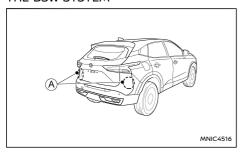
The Blind Spot Warning (BSW) system can help alert the driver of other vehicles in adjacent lanes when changing lanes.
