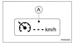
When pushing the Drive Assist switch on, the ICC system display and indicators are displayed in the vehicle information display. After you hold the Drive Assist switch for longer than about 1.5 seconds, the ICC system display goes out. The cruise indicator appears. You can now set your desired cruising speed. Pushing the Drive Assist switch again will turn the system completely off.
