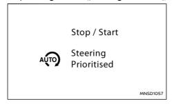
This guidance is displayed when the vehicle is stopped if the Stop/Start System is deactivated due to steering operation being detected.
