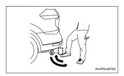
The tailgate can be operated using a guick kicking motion under the centre of the rear bumper.
