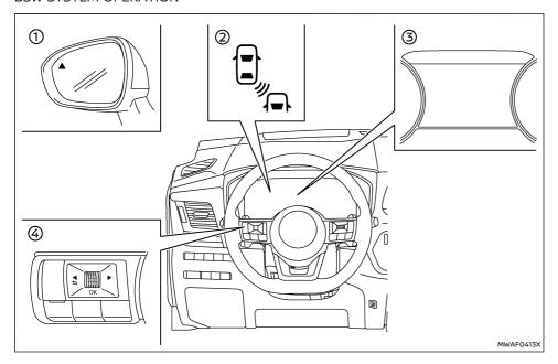
chimes (twice) and the BSW LED indicator light and the BSW indicator will flash. The BSW LED indicator light and the BSW indicator continue to flash until the detected vehicle leaves the detection zone.
