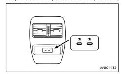
Two USB power ports (where fitted) are provided on the rear of the console box/armrest unit.
