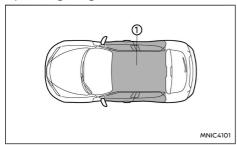
The Intelligent Key can only be used for starting the engine when the Intelligent Key is within the specified operating range (1) as illustrated.
