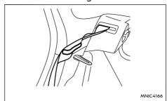
When folding the rear seat forward, the outer seat belts can be stored out of the way using the seat belt hooks as shown in the illustration.
