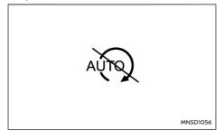
This indicator is displayed when the vehicle is stopped if the engine is prevented from automatically stopping by the Stop/Start System due to inhibition conditions.
