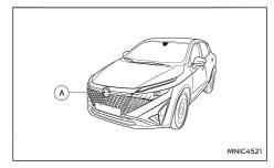
The I-FCW system uses a radar sensor (A) located on the front of the vehicle to measure the distance to a second vehicle ahead in the same lane
