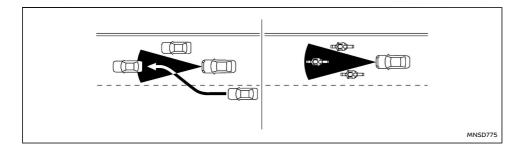
The detection zone of the radar sensor is limited. A vehicle ahead must be in the detection zone for the ICC system to maintain the selected distance from the vehicle ahead. A vehicle ahead may move outside of the detection zone due to its position within the same lane of travel. Motorcycles may not be detected in the same lane ahead.
