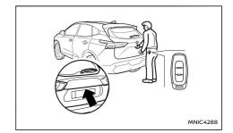
When the Intelligent Key is within the range of operation, the door locks can be locked or unlocked by pushing the door handle request button on the driver's or front passenger's door or the tailgate request button (where fitted).
