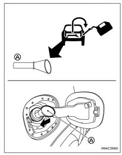
If you need to refuel from a portable fuel container, use the funnel (A) stored in the tool storage area (located under the luggage board).
