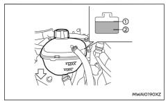
Check the coolant level in the reservoir when the engine is cold. If the coolant level is below MIN level 2), add coolant up to the MAX level (1).
