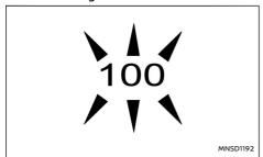
The driver can override ICC by pressing the accelerator. The set speed indicator will flash when the vehicle speed exceeds the set speed. The vehicle detect indicator will turn off when the area ahead of the vehicle is clear. When the pedal is released, the vehicle will return to the previously set speed.
