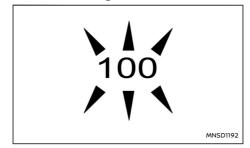
The driver can override ICC by pressing the accelerator. The set speed indicator will flash when the vehicle speed exceeds the set speed. The vehicle detection indicator will turn off when the area ahead of the vehicle is clear. When the pedal is released, the vehicle will return to the previously set speed.
