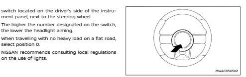
To sound the horn, push the centre pad area of the steering wheel.
