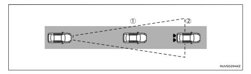
The I-FCW system operates at speeds above approximately 5 km/h (3 MPH).
