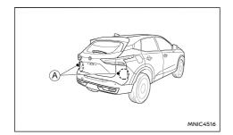
The RCTA system uses radar sensors (A) installed on both sides near the rear bumper to detect an approaching vehicle.
