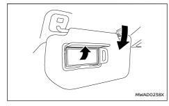
To use the vanity mirror, pull down the sun visor and pull up the cover. The memory seat system has the following features:
