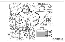
Check the coolant level in the reservoir when the engine is cold. If the coolant level is below the MIN
