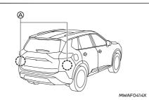
The two radar sensors A for the BSW system are located near the rear bumper. Always keep the area near the radar sensors clean.
