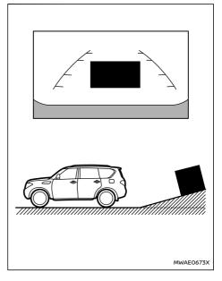
When reversing the vehicle up a hill, the distance guide lines and the vehicle width guide lines are shown closer than the actual distance. Note that any object on the hill is farther than it appears on the monitor.
