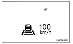
When passing another vehicle, the vehicle set speed indicator (a) flashes when the vehicle speed exceeds the set speed. The vehicle ahead detection indicator turns off when the area ahead of the vehicle is open. When the pedal is released, the vehicle returns to the previously set speed. Even though your vehicle speed is set in the ICC system, you can depress the accelerator pedal when it is necessary to accelerate your vehicle rapidly.
