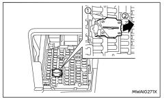
The extended storage switch is used when shipping the vehicle. It is located in the fuse panel. If any electrical equipment does not operate, ensure the extended storage switch is pushed fully in place.
