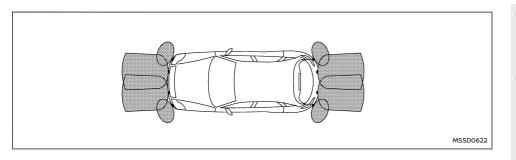
The parking sensor (sonar) system sounds a tone to inform the driver of obstacles near the bumper. When the parking sensor (sonar) system is turned on, the parking sensor (sonar) view will automatically appear in the vehicle information display.
