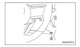
The sensors (1) and (2), located on the instrument panel, help maintain a constant temperature. Do not put anything on or around the sensors.
