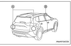
The two radar sensors (A) for the Intelligent Blind Spot Intervention system are located near the rear bumper. Always keep the area near the radar sensors clean. The radar sensors may be blocked by temporary ambient conditions such as splashing water, mist or fog.
