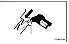
The fuel tank is not equipped with a fuel-filler cap. After opening the fuel-filler lid, insert the fuel pump nozzle directly into the fuel-filler opening. When the fuel pump nozzle is pulled out, the fuel-filler opening will be sealed.
