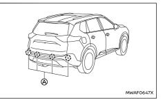
The parking sensors A are located on the rear bumper. Observe the following items to ensure proper operation of the system:
