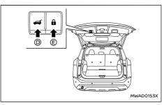
Power back door close and lock switches – Back door
