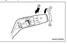
The rear window wiper and washer operate when the ignition switch is in the ON position.
