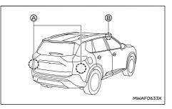
The Intelligent Blind Spot Intervention system uses radar sensors (a) installed near the rear bumper to detect other vehicles in an adjacent lane. In addition to the radar sensors, the Intelligent Blind Spot Intervention system uses a camera (b) installed behind the windscreen to monitor the lane markers of your travelling lane.
