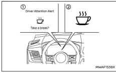
The system resets and starts reassessing driving style and steering behavior when the ignition switch is cycled from the ON to the OFF position and back to the ON position.
