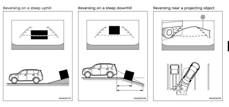
When reversing the vehicle up a hill, the distance guide lines and the vehicle width guide lines are shown closer than the actual distance. Note that any object on the hill is farther than it appears on the monitor. When reversing the vehicle down a hill, the distance guide lines and the vehicle width guide lines are shown farther than the actual distance. Note that any object on the hill is closer than it appears on the monitor.
