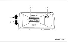
The speed limiter set switches are located on the steering wheel.
