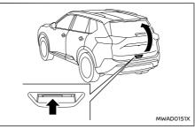
To open the back door, unlock it. Pull up the back door to open.
