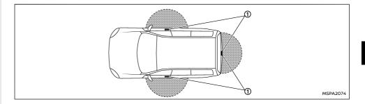
The Intelligent Key functions can only be used when the Intelligent Key is within the specified operating range from the lock or capacitive unlock sensors/request switch (f).
