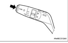
To turn off the adaptive LED headlight system, push the switch again.
