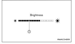
The instrument brightness control switch can be operated when the ignition switch is in the ON position. When the switch is operated, the vehicle information display switches to the brightness adjustment mode.
