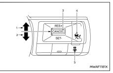
The system is operated by the Cruise ON/OFF switch and four control switches, all mounted on the steering wheel.
