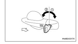
To lock the driver's door, turn the driver's door key cylinder to the rear of the vehicle (1).
