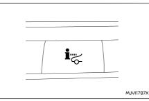
To turn the HUD on, push the HUD switch. To turn the HUD off, push the switch again.
