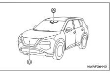
The radar sensor (B) is located on the front of the vehicle. The camera (A) is located on the upper side of the windscreen.
