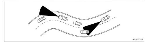
When driving on some roads, such as winding, hilly, curved, narrow roads, or roads which are under construction, the radar sensor may detect vehicles in a different lane, or may temporarily not detect a vehicle travelling ahead. This may cause the Intelligent Forward Collision Warning system to work inappropriately.
