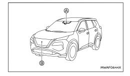
The Intelligent Emergency Braking with Pedestrian Detection system uses a radar sensor (B) located on the front of the vehicle to measure the distance to the vehicle ahead in the same lane.
