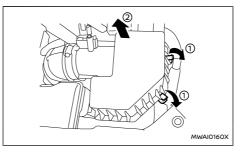
To remove the filter, release the lock pins (1) and pull the unit upward (2).
