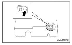
6. Place the ignition switch in the ON position. Then turn the compressor switch to the ON (-) position and inflate the tyre up to the pressure that is specified on the tyre placard affixed to the driver's side centre pillar if possible, or to the minimum of 180 kPa (26 psi). Turn the air compressor off briefly in order to check the tyre pressure with the pressure gauge.
