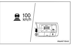
To set cruising speed, accelerate your vehicle to the desired speed, push down the **<CANCEL>**
