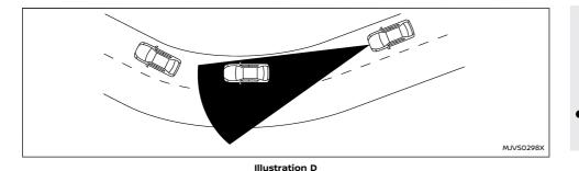
certain limitations. The system may not detect some forms of obstruction of the sensor area such as ice, snow, stickers, for example. In these cases, the system may not be able to warn the driver properly. Be sure that you check, clean and clear the sensor area regularly.
