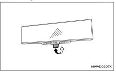
The mode can be switched when the ignition switch is in the ON position.
