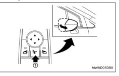
The outside rearview mirror remote control operates when the ignition switch is in the ON position.
