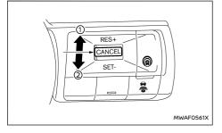
The vehicle set speed can be adjusted.
