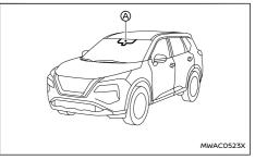
The ambient image sensor (A) for the high beam assist system is located in front of the inside rearview mirror. To keep the proper operation of the high beam assist system and prevent a system malfunction, be sure to observe the following:
