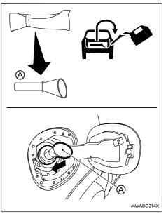
If you need to refuel from a portable fuel container, use the funnel (A) stored in the tool bag (located under the luggage board).
