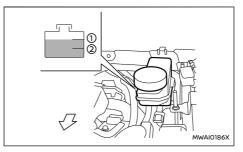
Check the fluid level in the reservoir. If the fluid is below the MIN line (2), the brake warning light will illuminate. Add fluid up to the MAX line (1). (See
