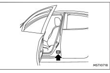
The vehicle identification plate is affixed as shown (on the driver's side).
