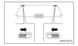
Before moving the rear (outer) luggage board, release the lock on the both sides of the board as shown (where fitted).
