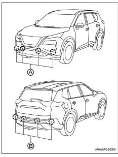
The parking sensors  $\textcircled{\sc B}$  (where fitted) and  $\textcircled{\sc B}$  are located on the bumpers.
