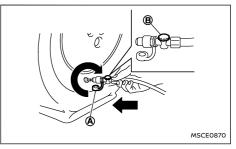
5. Remove the protective cap (a) of the hose and screw the hose securely onto the tyre valve. Make sure that the pressure release valve (b) is securely tightened. Make sure that the air compressor switch is in the OFF (c) position, and then insert its power plug into the power outlet in the vehicle.
