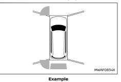
The parking sensor indicator also appears on the camera view of the centre display (where fitted).
