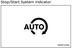
This indicator is displayed when the Stop/Start System is activated.
