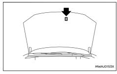
The air conditioner specification label is attached to the underside of the bonnet as shown.
