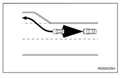
When driving on the highway at a vehicle set speed and approaching a slower travelling vehicle ahead, the ICC system adjusts the speed to maintain the distance, selected by the driver, from the vehicle ahead. If the vehicle ahead changes lanes or exits the highway, the ICC system accelerates and maintains the vehicle set speed. Pay attention to the driving operation to maintain control of the vehicle as it accelerates to the set speed.
