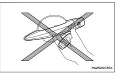
Do not use the lock or capacitive unlock sensors or request switch with the Intelligent Key held in your hand as illustrated. The close distance to the door handle will cause the Intelligent Key system to have difficulty recognising that the Intelligent Key is outside the vehicle.
