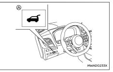
Power back door switch - Instrument panel
