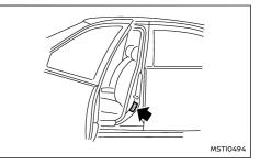
The cold tyre pressures are shown on the tyre placard affixed to the driver's side centre pillar.
