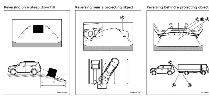
When reversing the vehicle down a hill, the distance guide lines and the vehicle width guide lines are shown farther than the actual distance. Note that any object on the hill is closer than it appears on the monitor.
