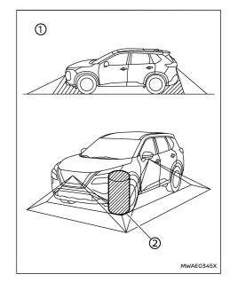
There are some areas where the system will not show objects and the system does not warn of moving objects. When in the front or the rear view display, an object below the bumper or on the ground may not be viewed ①. When in the bird'seye view, a tall object near the seam ② of the camera viewing areas will not appear in the monitor. The following are operating limitations and do not represent a system malfunction:
