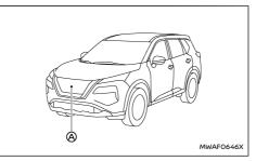
The Intelligent Forward Collision Warning system uses a radar sensor (A) located on the front of the vehicle to measure the distance to a second vehicle ahead in the same lane.
