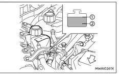
Check the coolant level in the reservoir when the engine is cold. If the coolant level is below the MIN level (2), add coolant to the MAX level (1).
