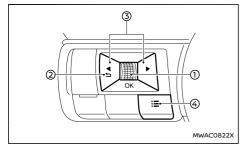
The vehicle information display can be changed using the scroll dial (1), 2 (2), and 4 (3) located on the steering wheel.
