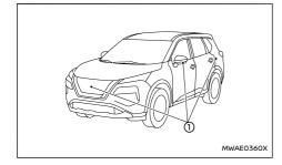
To display the multiple views, the Intelligent Around View Monitor system uses cameras () located on the front grille, on the vehicle's outside rearview mirrors and one just above the vehicle's rear number plate.
