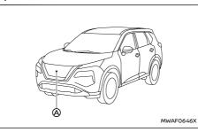
The sensor for the ICC system  $\textcircled{\ensuremath{\boldsymbol{\Theta}}}$  is located on the front of the vehicle.
