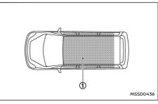
The Intelligent Key can only be used for starting the engine when the Intelligent Key is within the specified operating range (1).
