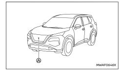
The radar sensor A is located on the front of the vehicle.
