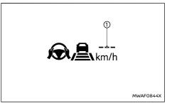
When the **<CANCEL>** switch is pushed down to **<SET->** under the following conditions, the ProPI-LOT Assist system cannot be set and the vehicle set speed indicator (1) blinks for approximately 2 seconds:
