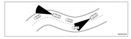
When driving on some roads, such as winding, hilly, curved, narrow roads, or roads which are under construction or on a slope, the sensor may detect vehicles in a different lane, or may temporarily not detect a vehicle travelling ahead. This may cause the system to work inappropriately.
