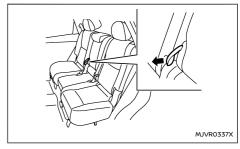
Pull the strap to unlatch the seatback and fold it down until it is horizontal.
