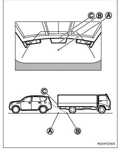
The position  $\bigcirc$  is shown farther than the position  $\bigcirc$  is actually. However, the position  $\bigcirc$  is actually at the same distance as the position O. The vehicle may hit the object when reversing to the position O if the object projects over the actual moving course.
