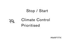
When the vehicle is stopped, the guidance is displayed if the Stop/Start system is deactivated since the air conditioner (cooling, heating or dehumidifying functions) is given priority.
